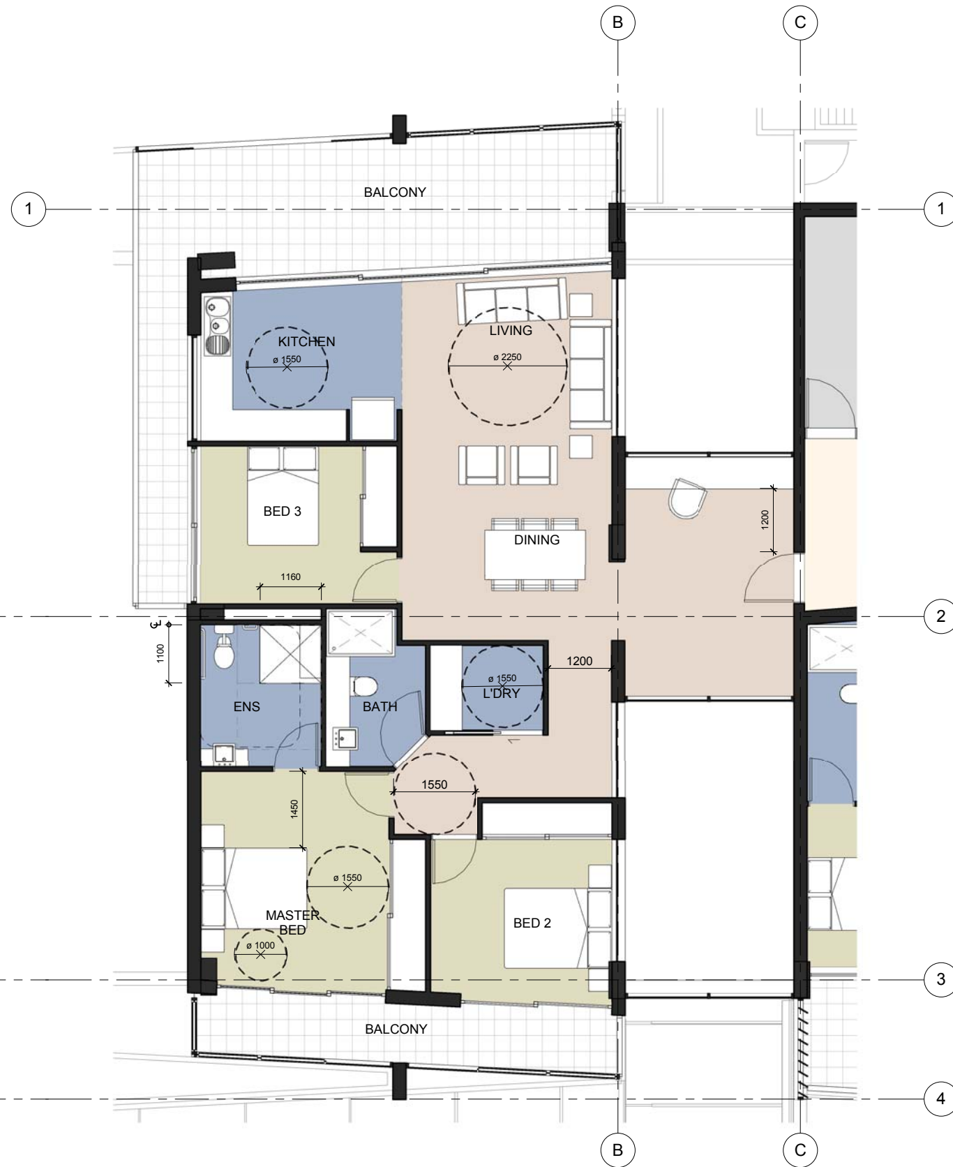
TYPICAL 3 BED ADAPTABLE UNIT- UNITS 82, 85, 88
