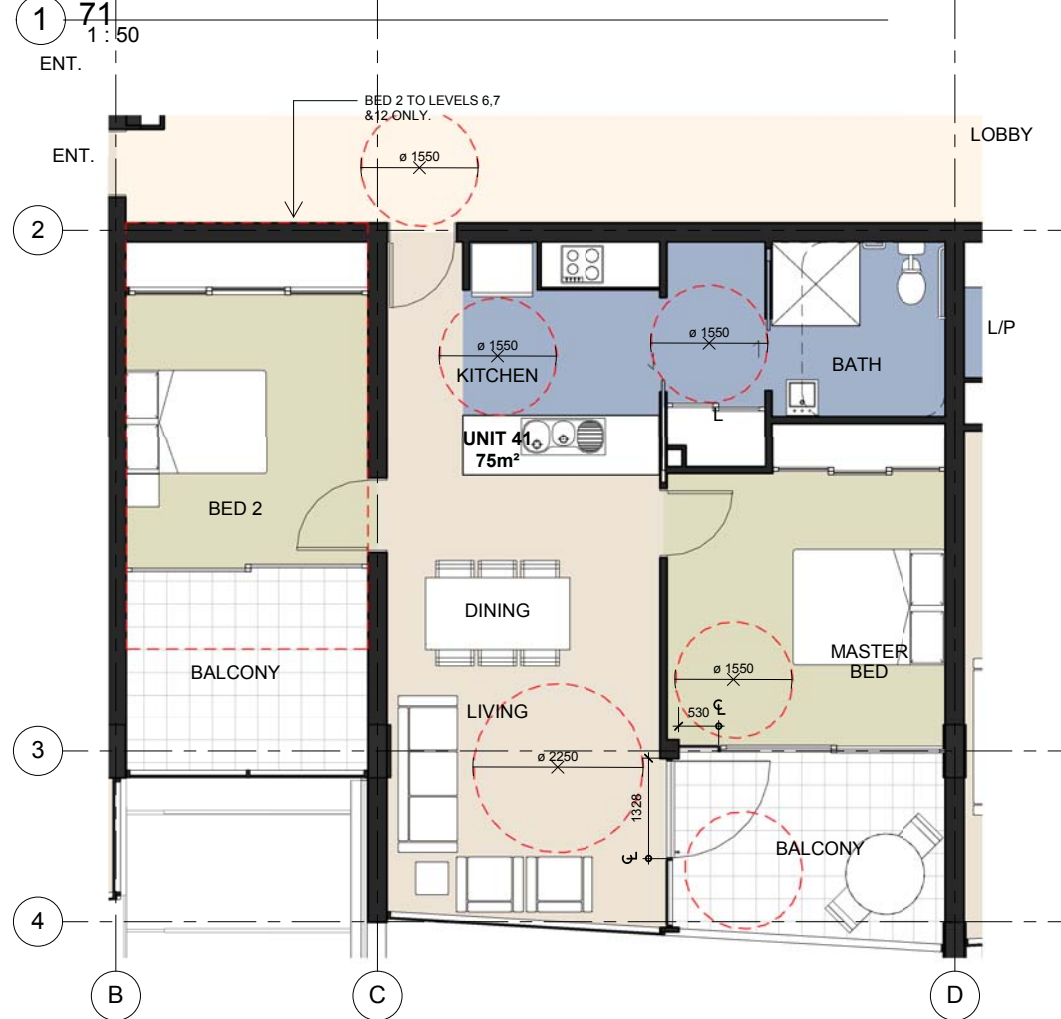
TYPICAL 2 BED ADAPTABLE UNIT- UNITS 41, 47, 77
